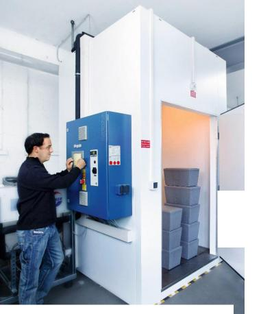
Storopack tests newly developed solutions for temperature-controlled shipping in the company's own environmental chamber.
