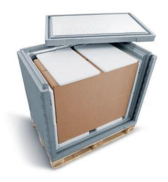
Thermoboxes are also available in the size of a Euro pallet (dimensions and internal volume of the box: 800 × 1,200 × 1,190 millimeters, 373.7 liters). These are ideal for transporting large volumes of temperature-sensitive products.
