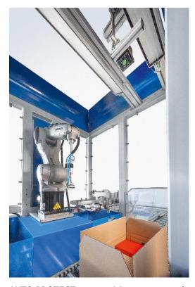
AUTO.PROTECT uses a vision system to detect voids in the box and determines the correct packing scenario using precise, trained AI. **Image: Storopack**
