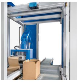
1. VOID DETECTION TO DETERMINE THE AMOUNT OF PROTECTIVE PACK-AGING MATERIAL REQUIRED
